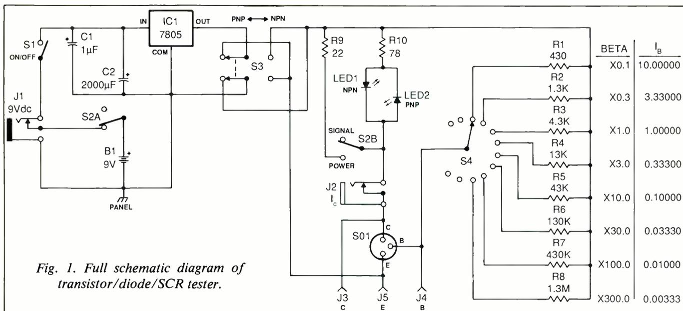
Fig. 1. Full schematic diagram of transistor/diode/SCR tester.
