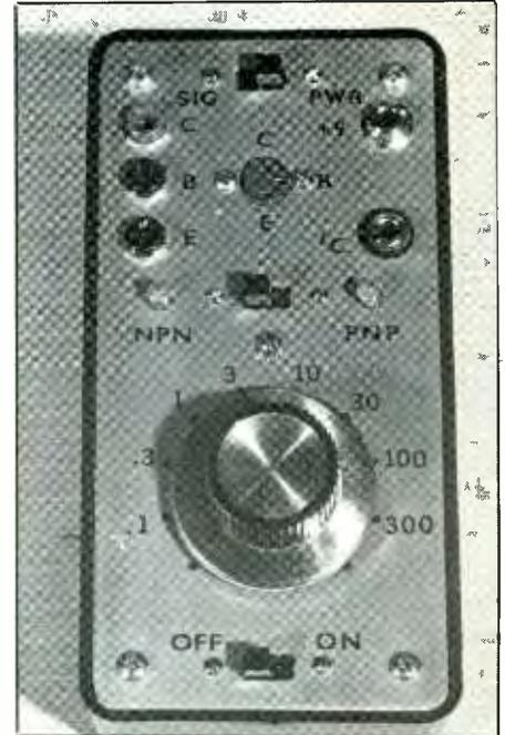
Fig. 3. Suggested front-panel layout, with appropriate panel labeling.
