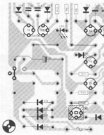
Unstabilised supply Tr = 18 V/100 mA C6 = 1000 \mu /25 V
