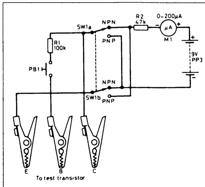
**Figure 1** Circuit diagram of the transistor tester
