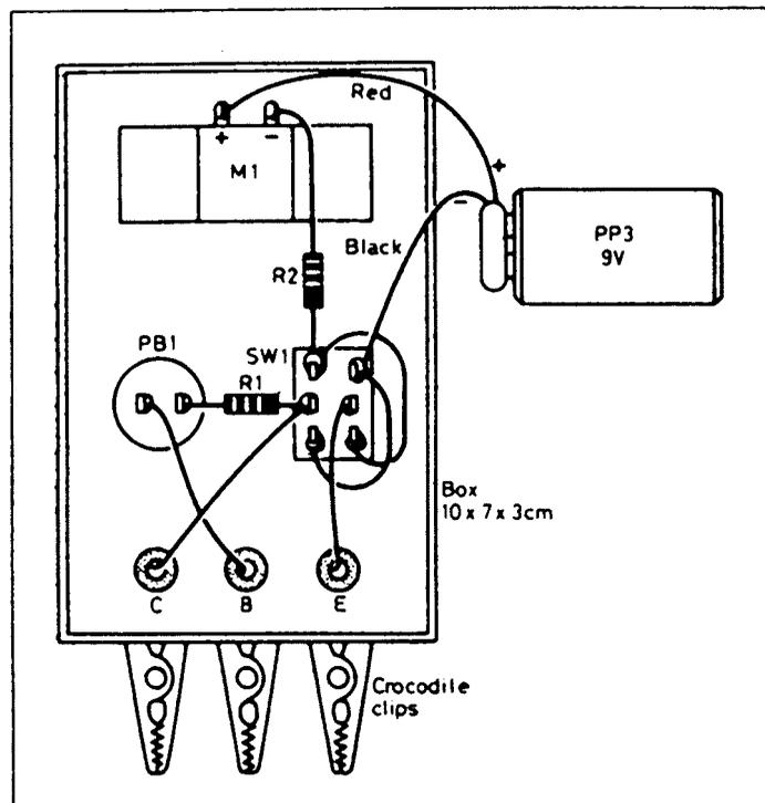
**Figure 3** This shows how to wire up the tester
