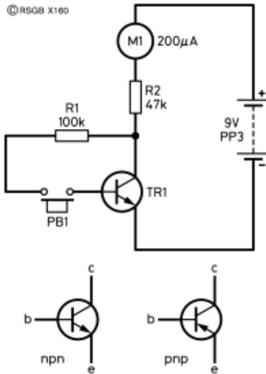
**Figure 2** Testing an npn transistor
