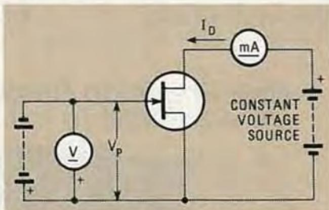
FIG. 9—MEASURE  $V_p$  by gradually increasing the gate voltage while monitoring  $I_D$ . When current stops increasing,  $V_p$  has been reached.
