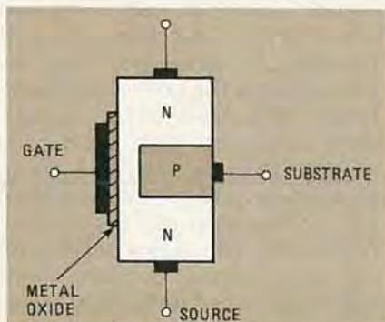
FIG. 6—MOSFET CONSTRUCTION is shown here. The oxide layer is usually silicon dioxide.
