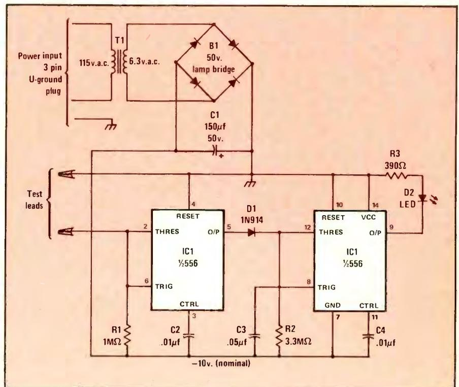
The potentiometer tester is built around a single 556 timer integrated circuit powered by a conventional full-wave bridge rectifier power supply. The circuit shown runs off the negative voltage output of the bridge. However, the circuit can be modified to operate from a positive dc voltage. The potentiometer or circuit under test is connected across the test leads.
