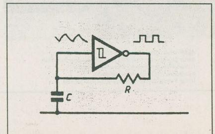
Fig. 3. Simplified Schmitt trigger inverter oscillator circuit.
