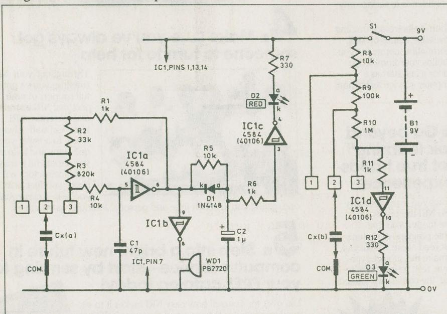
Fig. 4. Full circuit diagram for the tester.
