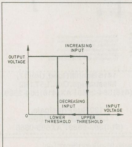
Fig. 2. Graph of the Schmitt trigger threshold levels.
