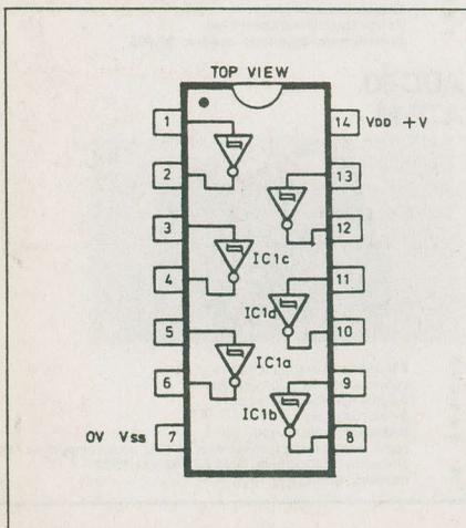
Fig. 1. The 4584 (40106) Hex Schmitt Trigger pinout details.
