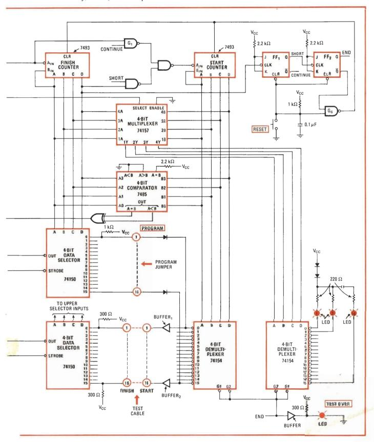
open circuit with a single numbered light-emitting diode, or a short circuit by lighting two numbered LEDs. The right branch of the flow chart shows this process.
