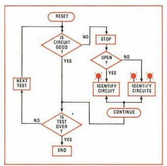
1. Finding cable faults. Flow chart summarizes the operation of a programable cable tester that can check out cables containing 16 or fewer circuits. Each circuit is tested for continuity, and all possible circuit combinations are checked for shorts. The tester is programed simply—by means of wire jumpers at the terminals.
