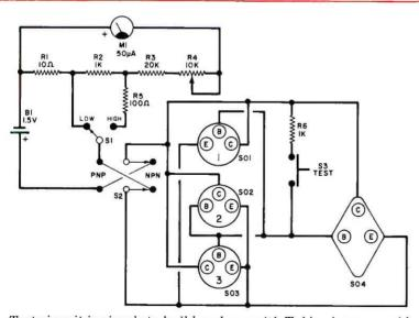
Test circuit is simple to build and use with Table above as guide.
