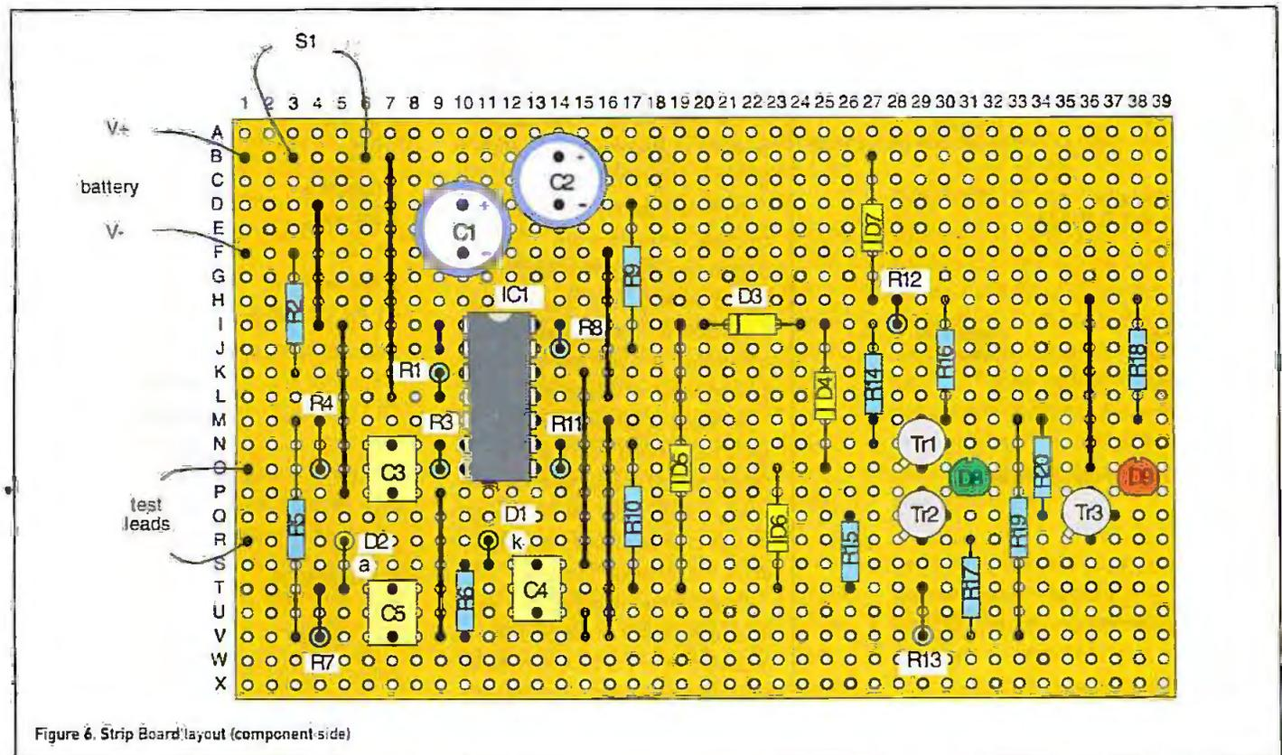
Figure 6. Strip Board layout (component side)
