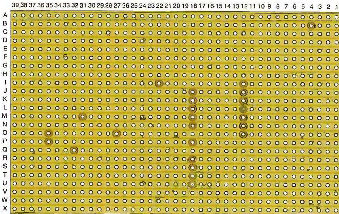
Figure 7. The Track Cuts Required On The Strip Board Layout (track side view).
