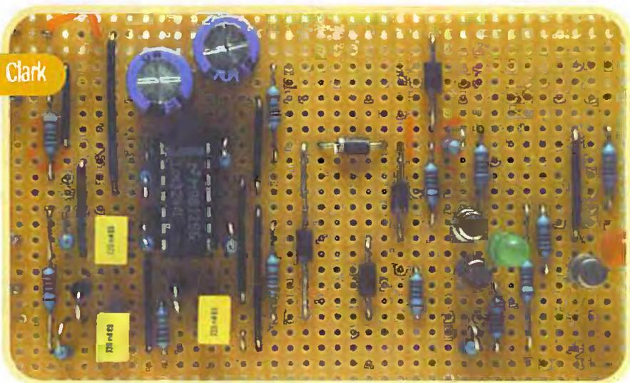
There's no need to mess about swapping leads to test the conduction in both directions, and no more having to guess whether the p-n junction is operating correctly by deciphering the resistance reading on a multimeter. This device will test whether or not a diode does just what a diode is supposed to do - rectify.
