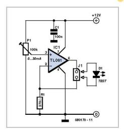
LEDs. If you wish, you can connect a multimeter across the LED to measure the voltage on the LED.
