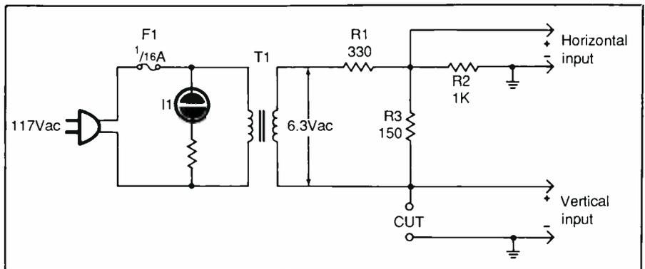
Fig. 1. Overall schematic diagram of In-Circuit Component Tester.
