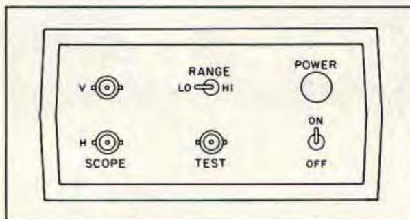
Figure 3. Front panel component layout.
