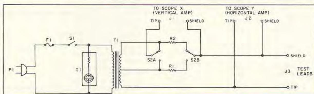
Figure 2. Schematic diagram for dynamic component tester.
