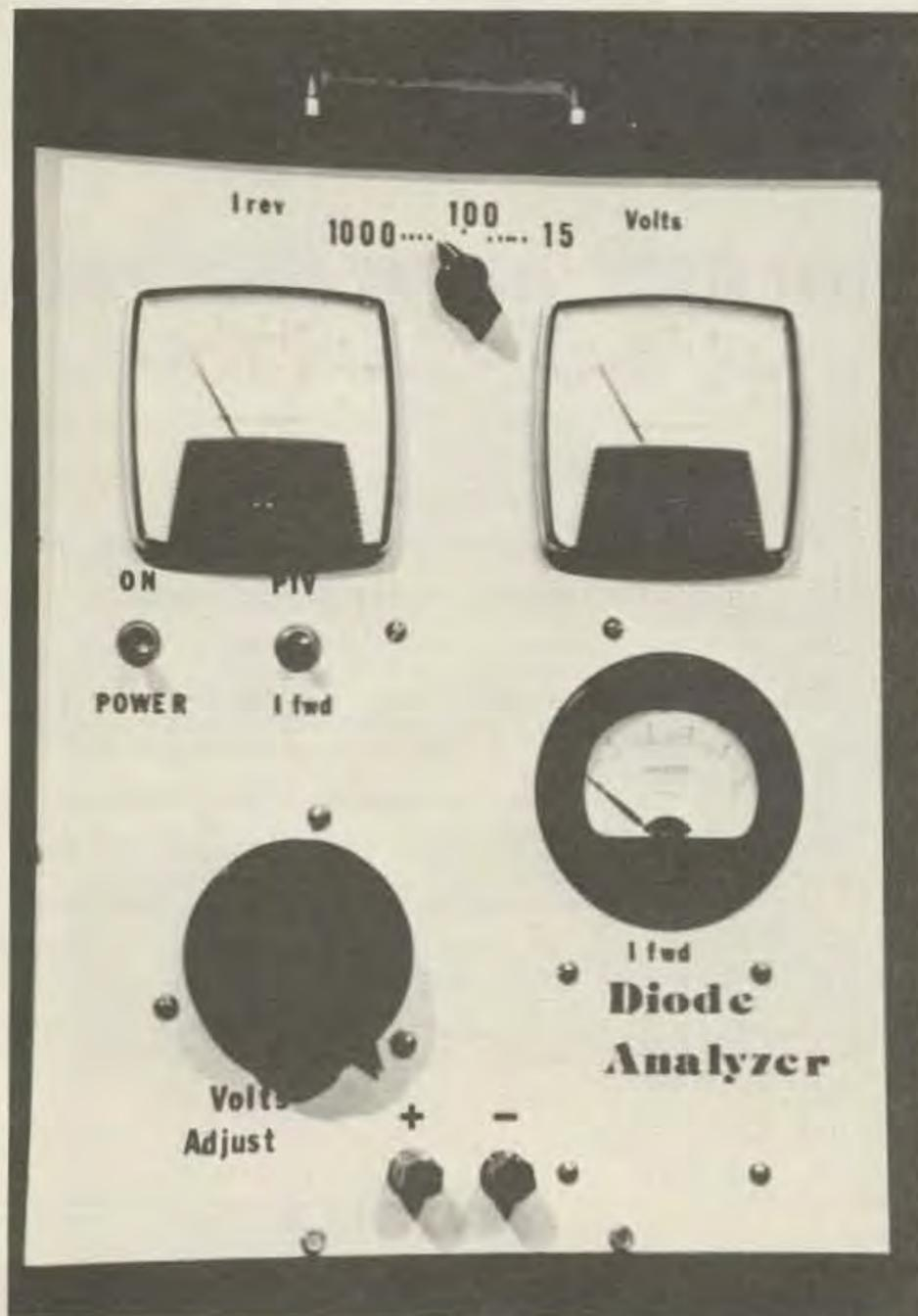
Front panel of the diode analyzer.
