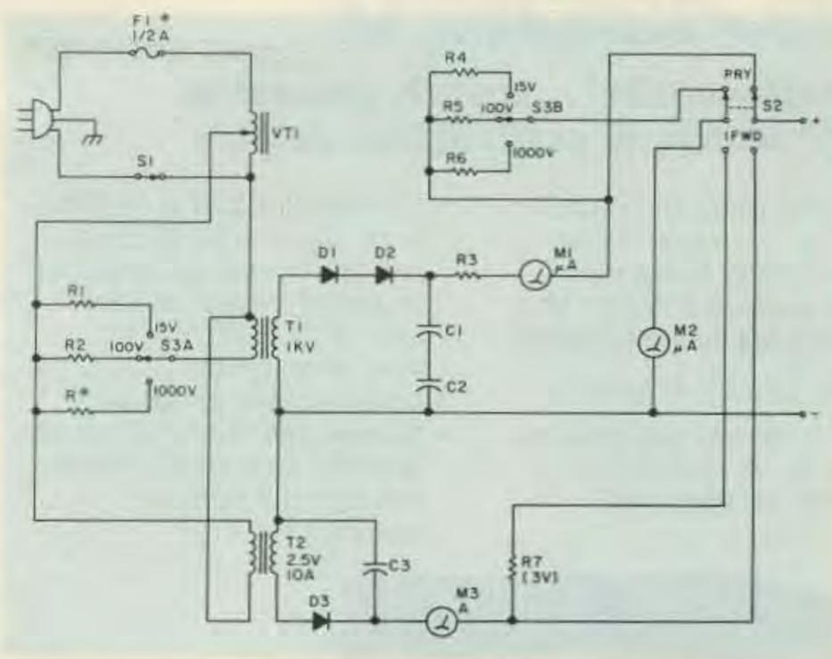
Fig. 1. The diode analyzer schematic diagram.
