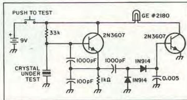
Figure 1. Original crystal tester circuit.
