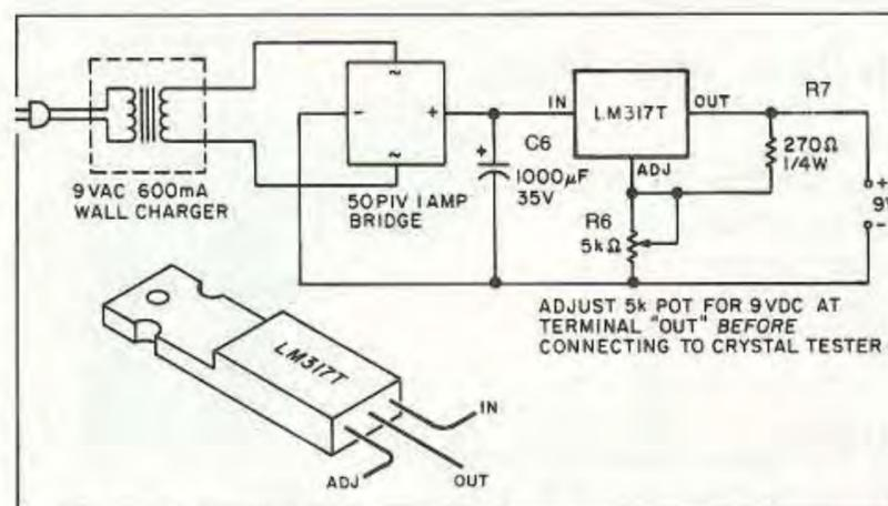
Figure 3. AC power supply for the crystal checker.
