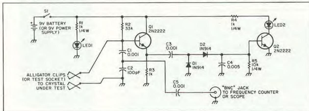
Figure 2. The improved crystal tester.
