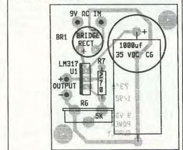
Figure 5. Parts placement.
