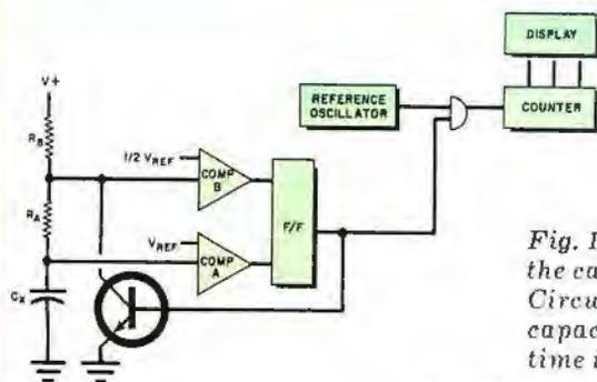
Fig. 1. Block diagram of the capacitance meter. Circuit determines unknown capacitance by measuring time it takes to discharge.
