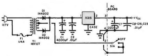
Fig. 6. Power supply circuit has a voltage regulator IC.
