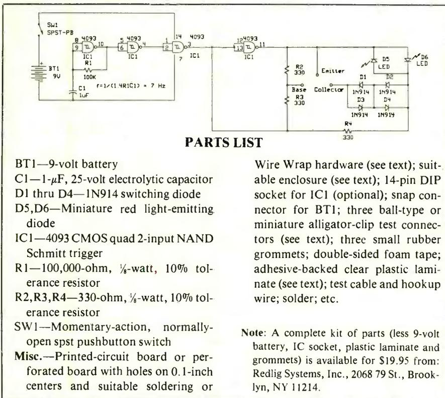
Fig. 1. Complete schematic diagram of In-Circuit Transistor Tester.
