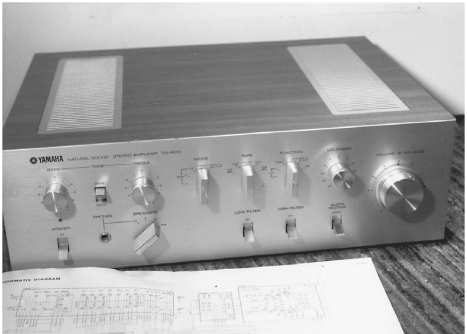
9-18 Check all electrolytic capacitors within the high-powered transistor stereo amplifier with an ESR meter.
