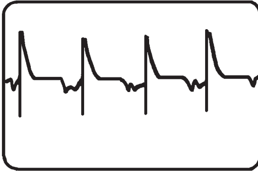
7-20 The horizontal driver transistor waveform indicating that the deflection and driver transistors are okay.
