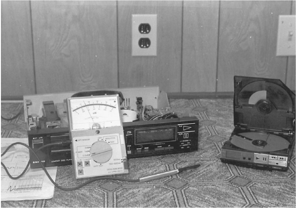
12-4 A laser power meter can quickly test a remote transmitter.
