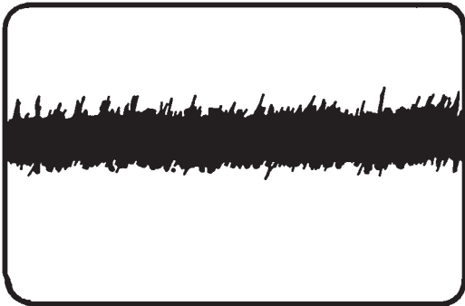
6-41 A tracking gain waveform taken across the tracking coil winding.
