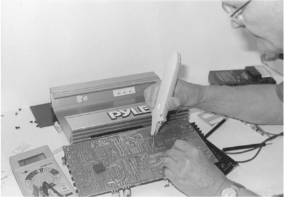
3-34 A typical high-powered 2 \times 350 -W Pyle amplifier that connects to a 2-ohm speaker load.
