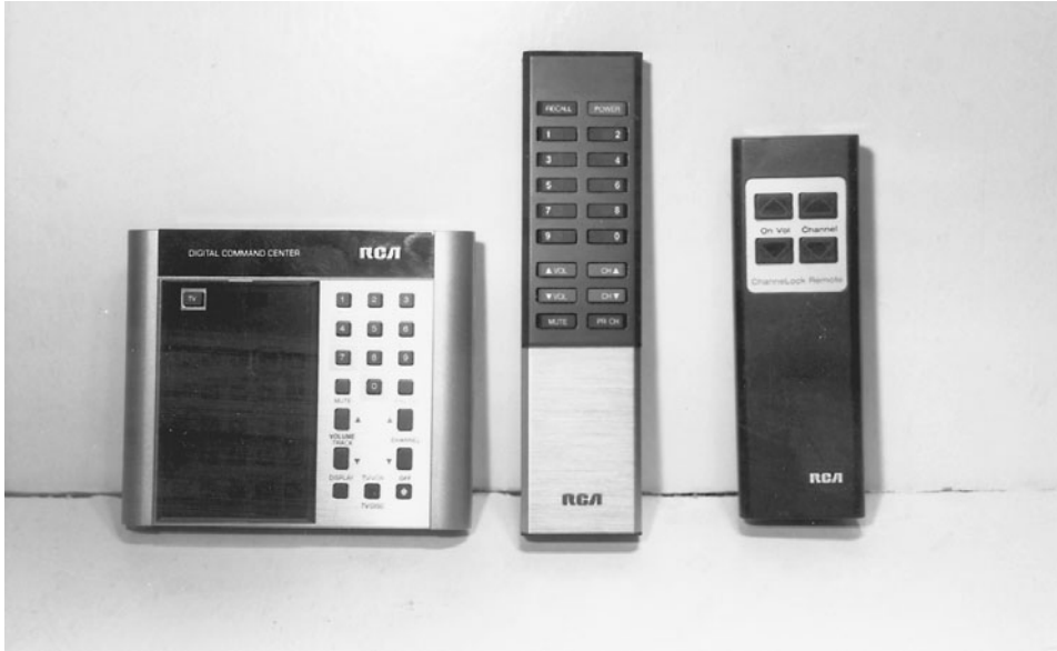
12-1 Early remote transmitters used RF control until the infrared remote was introduced.
