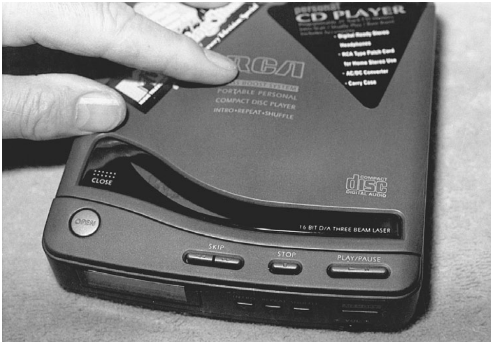
6-22 The door or lid must be closed on a portable CD player before the CD will spin.
