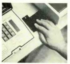
the pad and the nearest electrical ground.) Prior to touching the computer or its accessories, I brush my fingers against the pad, instantly discharging any static voltage I might have accumulated. The conductive foam is the stuff used to store or ship integrated circuits. Many electronics shops sell small sections, or will give the scraps away at no charge.
