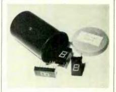
vices, like other DIP chips, are prone to pin damage when stored in a bigger container where the weight of other parts will bend the pins. Also, with the lid of the container marked to indicate the contents, the experimenter will have no trouble finding the desired part quickly!
