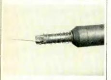
Plug the iron in, and after a few minutes you'll have a *needle-point* soldering tip suitable for delicate repairs. To prevent the wire tip from moving backward when pressed against a connection, stretch the spiral so that the end is right up against the body of the soldering iron. The spiral serves as a spring, producing a slight *give* as the tip is pressed against the foil surface.
