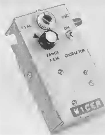
Fig. 70 — Exterior view of the test unit. A small Minibox serves as a case.
