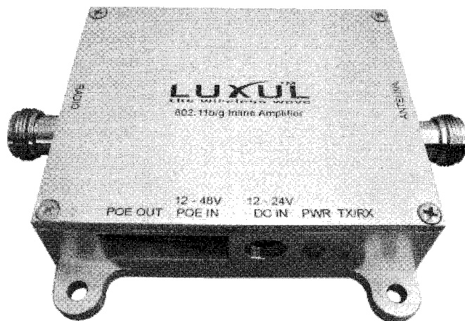
Figure 7-8 —A typical bi-directional amplifier for HSMM applications. This unit delivers 1 W output.
