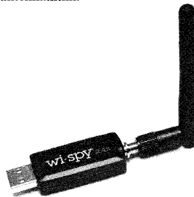
Figure 7-6 —This 802.11 b/g Wireless LAN USB Adapter features an external RP-SMA female connector if you wanted to extend its range with an optional antenna. Transmit power is a standard 15dBm. It is perfect to travel with and it is the size of a removable USB Thumb Drive, so you can keep it in your pocket!
