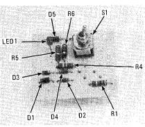
FIG. 6---THE COMPLETED PC board is shown here.
