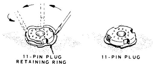
HOLD THE PLUG IN THE CHASSIS HOLE AND PLACE ONE END OF THE RING INTO THE GROOVE OF THE PLUG. USING A SCREWDRIVER, PRESS THE RING INTO THE GROOVE AROUND THE PLUG.
