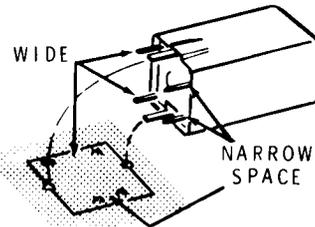
NOTE: Use a minimum of solder in the following steps to prevent rosin from getting into the control.
