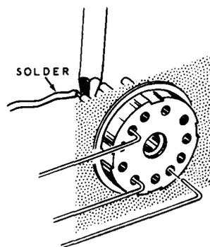
① PUSH THE WIRE INTO THE HOLE UNTIL IT COMES OUT OF THE END OF THE PIN
