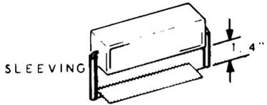
( ) 2500  $\Omega$ , 7-watt (2.5 k $\Omega$ ). Use 1/2" of small black sleeving on each lead as above.
