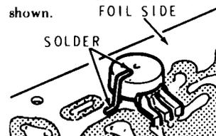
( ) Check to see that all connections are soldered before putting the board aside. Disregard any unused holes.
