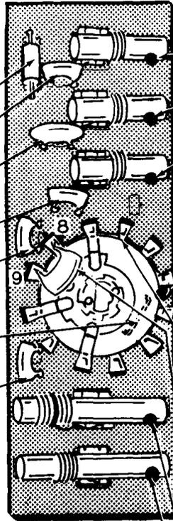
NOTE: Solder the pins of the coils and switch wafer as they are installed, but do not cut off their pins after soldering.
