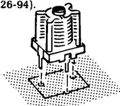
( ) Install a 7-pin tube socket at V2.
