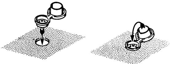
POSITION THE SMALL PORTION OF THE GROMMET INTO THE CHASSIS HOLE.
