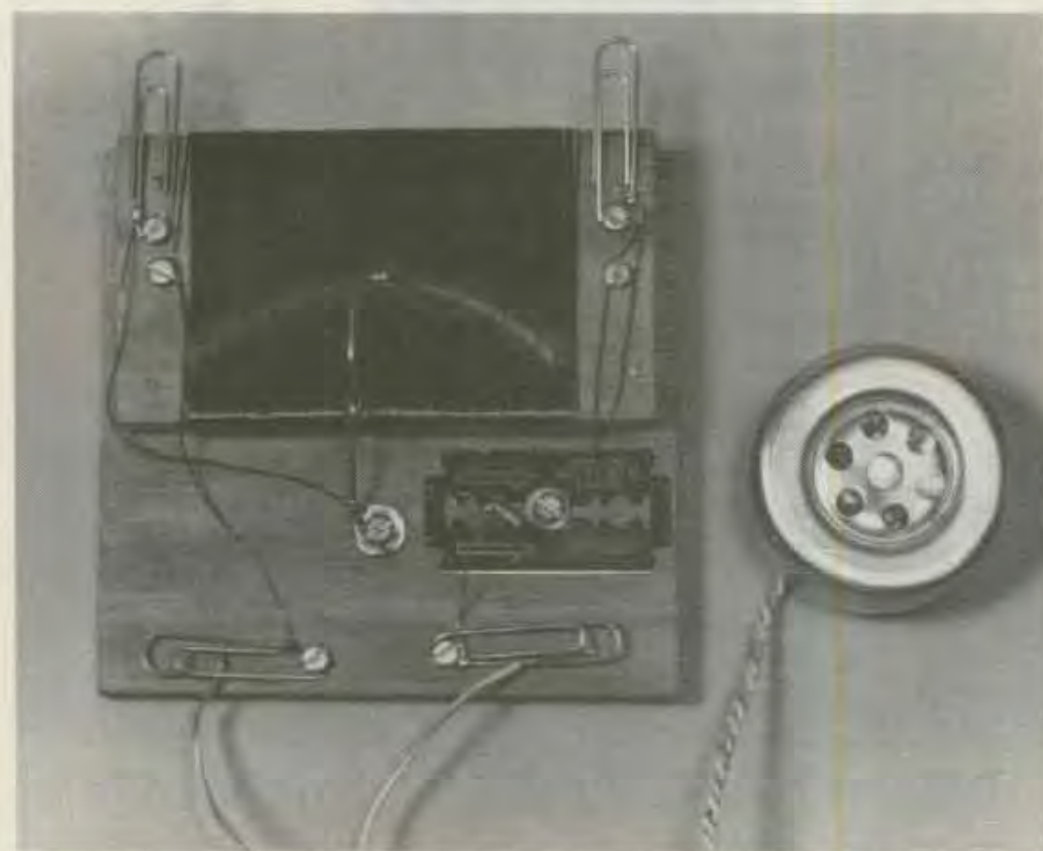
Photo A. A close replica of a set W8EFW described in 1945, this Foxhole radio can be built for pennies and works amazingly well. The razor blade is the diode. The earphone was borrowed from a telephone.
