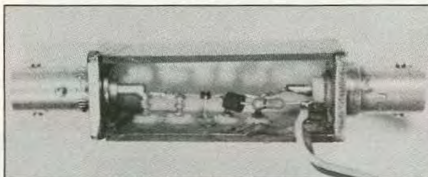
Photo A. Close-up of the finished amplifier: MAR-8 (center), chip caps, resistor, stand-off insulator bead on the resistor lead, BNC connectors and 12 volt wires.
