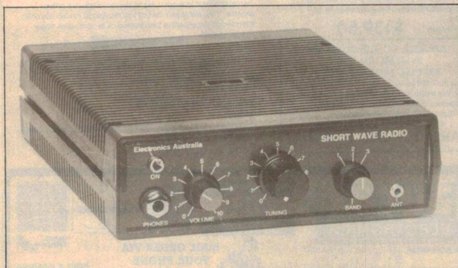
The front panel controls are for volume, tuning and band switching.
