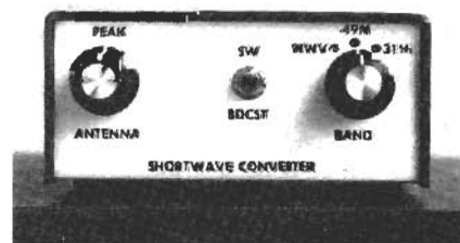
FIG. 7—THE COMPLETED CONVERTER. If you wish, follow the design shown here when laying out your front panel.
