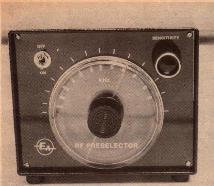
An aluminium case was used to house the prototype.
