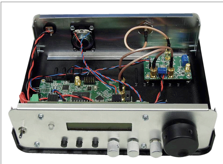
Figure 4. A look inside our finished prototype. Notice how the antenna input cable loops to accommodate its slightly too great length.
