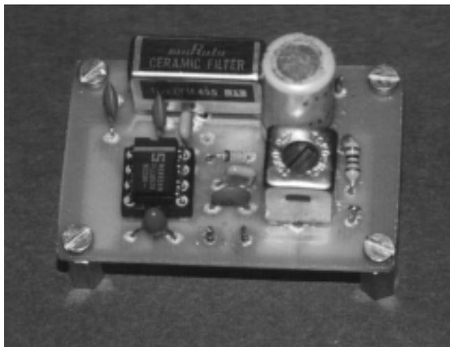
The superhet is far more sensitive than the direct-conversion type, and can weed out those elusive DX stations. You may have found that a station will appear at two places on the dial of the direct-conversion receiver; you will have no such problem with the superhet.
