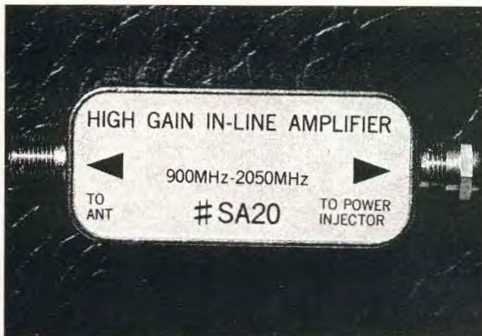
Photo D. A masthead amplifier sold for the satellite TV market is used.
