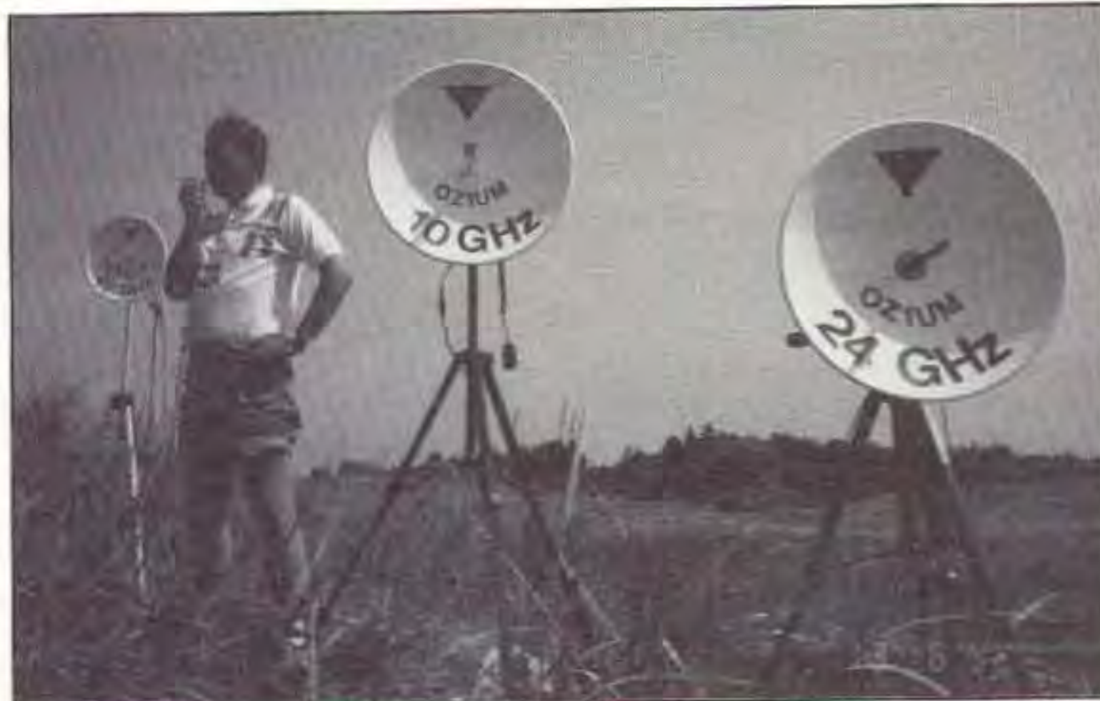
Photo A. OZ1UM with his microwave setup in Denmark for 10, 24, and 47 GHz operation.
