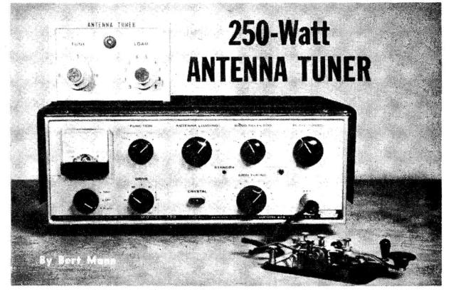
MANY amateurs working 40 or 80 meters don't have enough room for a half-wave antenna and must settle for a random length of wire. While a random-length job will radiate some RF, the full get-out ability of the transmitter rarely is realized.
