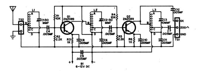
R1,R4—10,000 ohms resistor, ½ watt, 10%, R2,R5—2,200 ohms resistor, ½ watt, 10%, R3,R6—1,000 ohms resistor, ½ watt, 10%, C1,C2,C3—2-30 mmf trimmer capacitor C4 to C12—.005 mf low-voltage ceramic discs or .0047 mf tubular types
