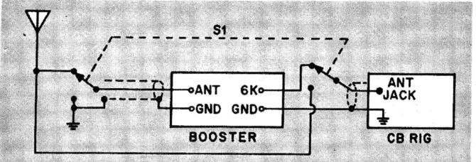
To protect the Booster during transmission periods, a double-pole, double-throw slide switch is required in addition to the transceiver's normal P-T-T switch. See text for specific details.
