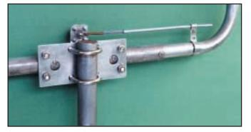
Figure 3—Gamma tuning assembly and mounting system. Two 1/2 inch holes are drilled through the aluminum mounting plate to clear the screw heads when the antenna is in the vertical plane.
