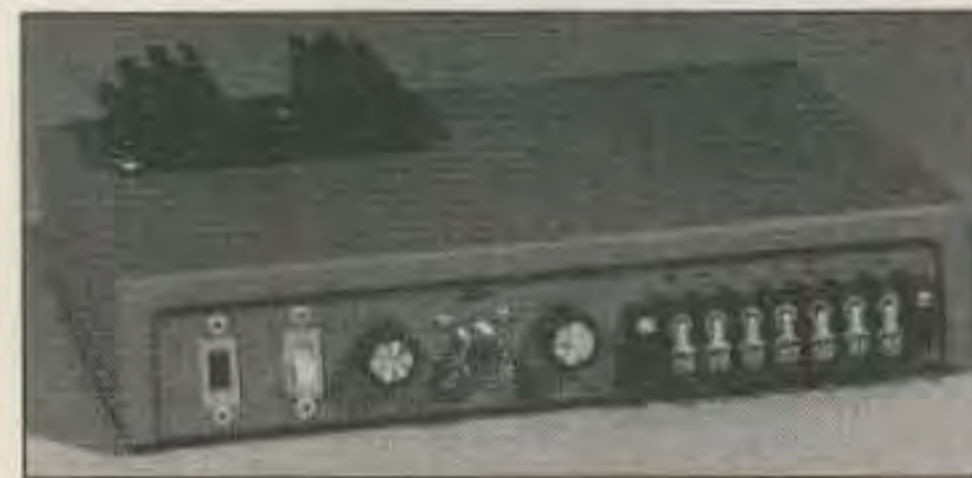
Photo C. Hidden transmitter in enclosure with heat sink for continuous duty operation.
