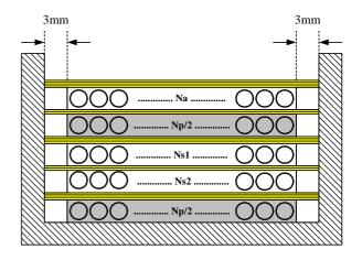
Figure 13. Sandwich winding
