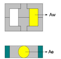
Figure 2. Window Area and Cross Sectional Area
