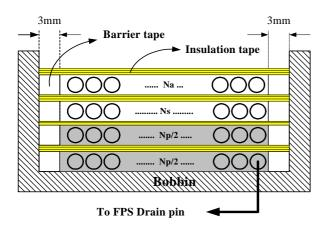
Figure 7. Primary side winding
