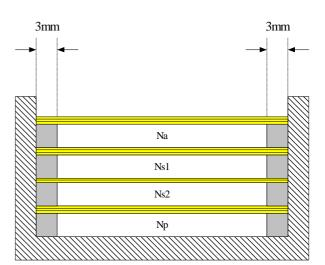
Figure 18. LCD monitor SMPS transformer construction example (B)
