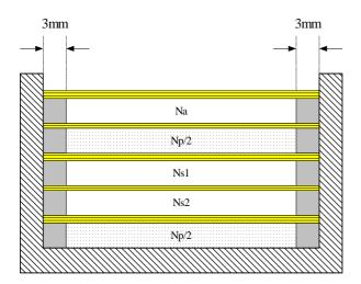
Figure 17. LCD monitor SMPS transformer construction example (A)
