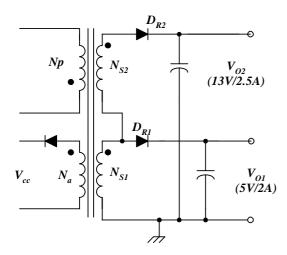
Figure 16. LCD monitor SMPS transformer example
