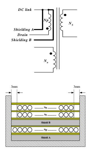
Figure 14. Shielding example to remove Y-capacitor
