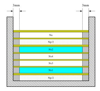
Figure 22. CRT monitor SMPS transformer construction example (SSR)
