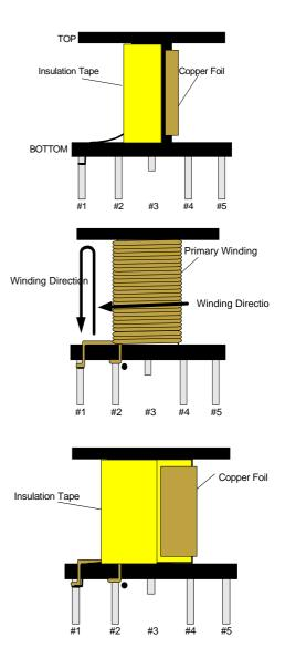
Figure 15. Shielding method to remove Y-Capacitor
