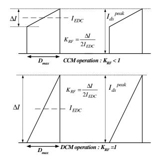
Figure 4. MOSFET Drain Current and Ripple Factor (K<sub>RF</sub>)
