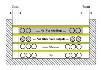
Figure 9. Winding sequence to reduce Vcc variation
