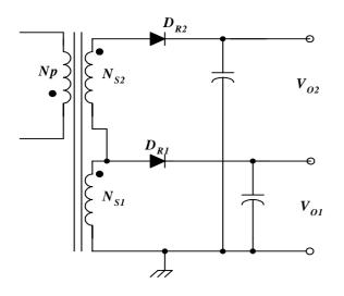
Figure 11. Stacked winding on other winding
