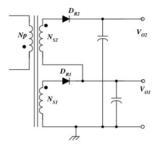
Figure 12. Stacked winding on other output
