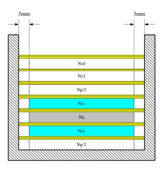
Figure 20. CRT monitor SMPS transformer construction example (PSR)
