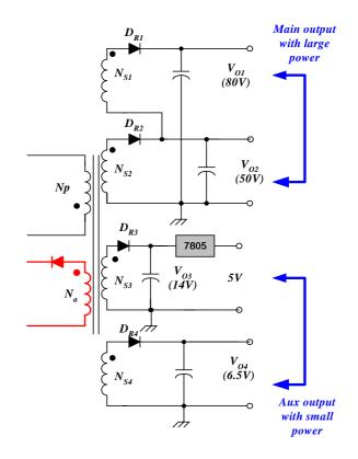
Figure 19. CRT monitor SMPS transformer example-PSR
