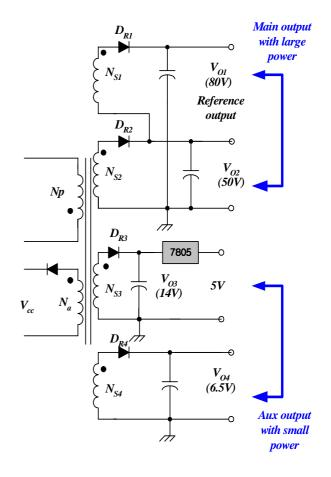
Figure 21. CRT monitor SMPS transformer example-SSR
