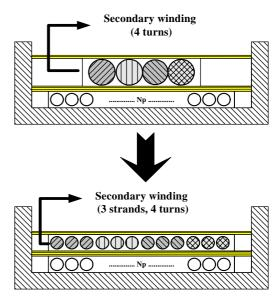
Figure 10. Multiple parallel strands winding
