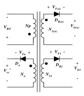
Figure 6. Simplified diagram of the transformer
