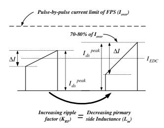
Figure 5. Adjustment peak drain current
