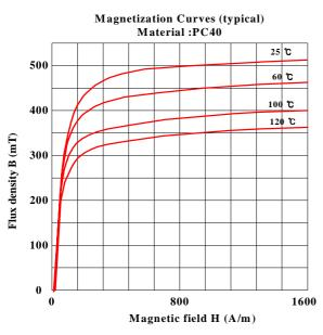
Figure 3. Typical B-H characteristics of ferrite core (TDK/PC40)
