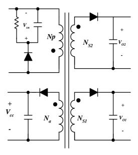
Figure 8. Primary side winding
