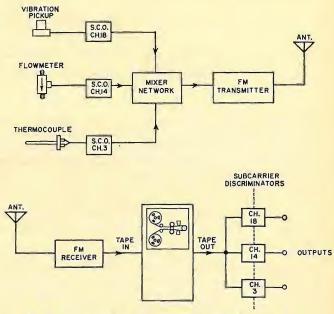
Fig. 3. A number of transducers may be multiplexed on signal.
