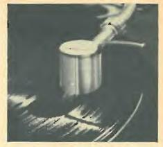
Operational theory of the cartridge is as follows: 1. the movement of the screen controls the amount of light ray passing through the screen on to the diode; 2. the movement of the stylus on the record causes the screen to vibrate; 3. the amount of light ray passing through the screen on to the diodes changes the current of the diodes to sound current. The cartridge, according to its maker, can transform the most minute vibration to electricity. Kenwood Circle No. 17 on Reader Service Card
