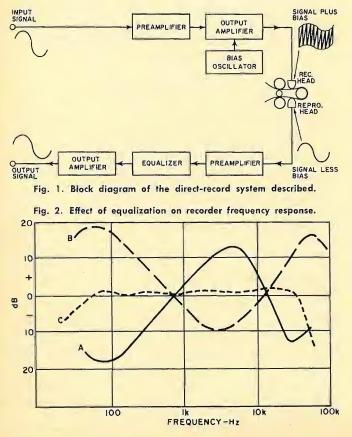
The reproduce signal at the playback head is shown minus the bias oscillator signal. Most of this is lost due to the spacing of the reproduce head gap. It is not sufficiently small so as to reproduce the high-frequency bias signal. The remainder of the bias signal is usually removed by a simple *RC* filter.
