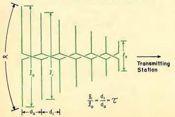
rections. In contrast, a directional antenna achieves gain in one direction at the expense of gain in all other directions. Since only noise signals would be received from the other directions anyway, you "get something for nothing". Therefore, a directional antenna improves the signal-to-noise ratio in two ways: the signal level is increased and the noise level is reduced by directional discrimination.
