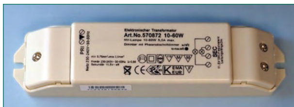
Figure 1. An off-the-shelf 'electronic transformer' providing 60 W of power for low-voltage halogen lamps.
