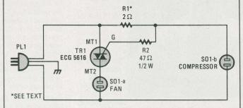
Fig. 6. When this Triac circuit senses current flow through SOIa, it activates the device plugged into SOI-b. The values of the resistors must be chosen for the specific devices to be plugged in.
