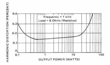
Figure 5-47 - 50-W-Amplifier Harmonic Distortion versus Output Power
