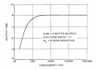
Figure 5-22 - Frequency Response Curve
