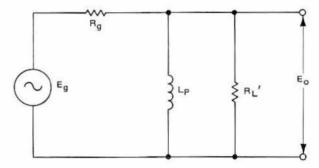
Figure 5-5 - Low-Frequency Equivalent Circuit of Transformer Coupling
