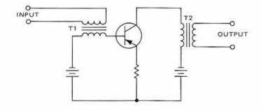
Figure 5-2 - Typical Class-A Amplifier
