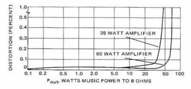
Figure 5-38 – Intermodulation Distortion (60 Hz & 7 kHz Mixed 4:1) versus Power Output
