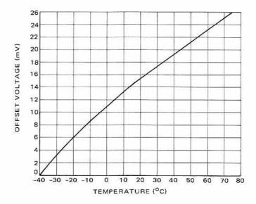
Figure 5-16 - DC Servo Amplifier Offset Voltage versus Temperature
