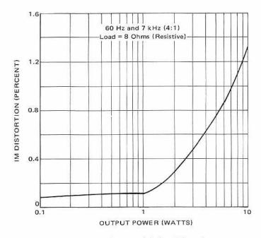
Figure 5-31 - Intermodulation Distortion
