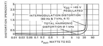
Figure 5-36 — Linearity and Clipping Characteristics
