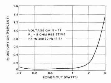
Figure 5-23 - IM Distortion versus Power Output
