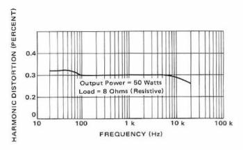
Figure 5-46 - 50-Watt-Amplifier Harmonic Distortion
