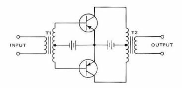
Figure 5-3 - Typical Class-A Push-Pull Amplifier
