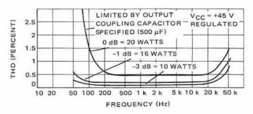
Figure 5-35 – Distortion versus Frequency Response
