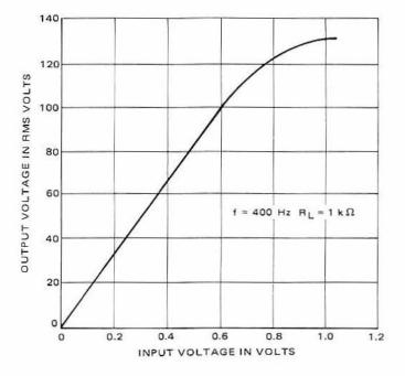
Figure 5-12 - Output Voltage versus Input Voltage
