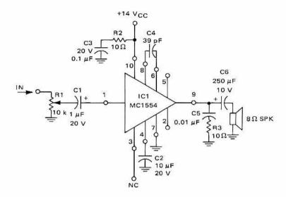
Figure 5-18 - 1 W Integrated Circuit Audio Amplifier
