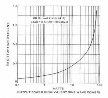
Figure 5-45 - 50-Watt-Amplifier Intermodulation Distortion
