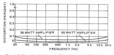
Figure 5-39 — Total Harmonic Distortion versus Frequency @ Rated Output to 8 Ohms
