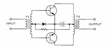
Figure 5-4 - Typical Class-B Push-Pull Amplifier
