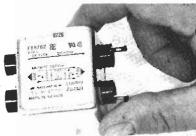
FIG. 2—THIS RF FILTER keeps RF power-line interference from leaking into your computer, and keeps your computer from interfering with other devices. It is particularly good at keeping two computers on the same power line from interfering with each other.
