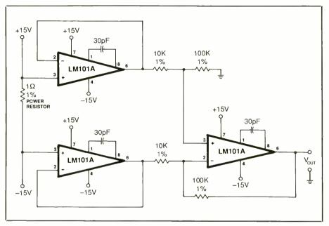
Fig. 1. Schematic diagram of a basic solid-state substitute current shunt.
