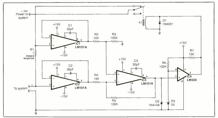
Fig. 2 Schematic diagram of the complete Substitute Cur rent Shunt circuit, including the relay switching circuit that automatically interrupts power to the protected system when excessive current is drawn and restores power when conditions return to normal.
