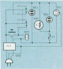
FIG. 1—THIS EASY-TO-BUILD CIRCUIT can provide better power-line protection for a personal computer than many commercial devices costing as much as \$150.
