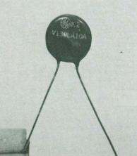
FIG. 3.—IT LOOKS LIKE A DISC CAPACITOR, but it's really a metal oxide varistor that limits transient line-voltage surges to about 180 volts.
