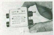
FIG. 2—THIS RF FILTER keeps RF power-line interference from leaking into your computer, and keeps your computer from interfering with other devices. It is particularly good at keeping two computers on the same power line from interfering with each other.
