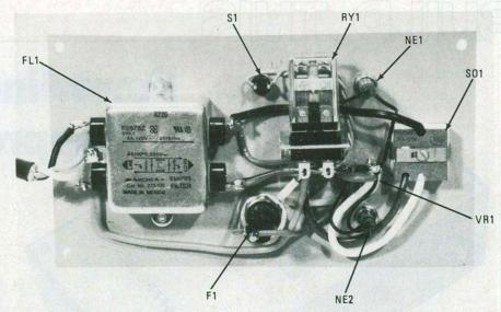
FIG. 4—ALL OF THE COMPONENTS mount on the metal front panel of a plastic utility cabinet.
