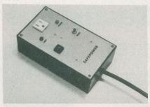
My two units (for two computers) are built inside a surplus Executone telephone desktop machine. I made two small additions: a) added MOV's from "hot" 115-volts AC to ground and from "neutral" to ground, to guard against transients. b) added a 4-amp fuse in series with the power-input line.
