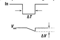
These waveforms define voltage droop  $(D_V)$ , the decline of capacitor voltage due to discharge during a time interval  $D_T$ .
