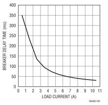
Figure 2. Low Current Transients Must Last Relatively Longer to Trip the Breaker. Higher Currents Trip the Circuit Breaker in Less Time
