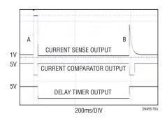
Figure 3. An Example Trip and Retry Sequence. At Time Point A, the 5A Load Current Spike Trips the Comparator and 60ms Later the Breaker is Opened. At Time B, After a Delay Time of 1.3 sec, the Timer Closes the Breaker. The Resulting Short Duration Spike of Start-Up Current Is Not Large Enough or Long Enough in Duration to Trip the Breaker Again
