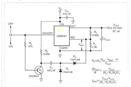
Figure 1 On power-up, the control current through  $R_{a}$ ,  $C_{y}$ , and  $D_{z}$  delays the rise of  $V_{OUT}$  and thus prevents excessive  $I_{MAX}$  transients.
