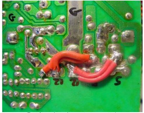
Transformer low voltage outputs are cutted, and 12 volt output vindings are connected to the high current double diode.
