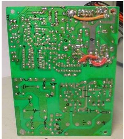
Orange wire connects unused cap to the new 13.5 Volt output (old +5 Output).
