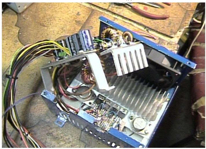
Normal mains 250 watt ATX power specifications. 3.30v @ 14A. 5.0v @ 22A. 12.0v @ 8A. 5.0 v SB @ 0.8A. -5.0v @ 0.3A. -12.0v @ 0.8A
