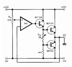
When working with i.cs it is often necessary to have positive and negative supplies, and it is desirable that each supply remains steady with changes in load current. This circuit has been a useful addition to an adjustable 0 to 15V stabilized supply. For +5 and -5V, potentiometer  $R_1$  is set to the mid position and the current through the output transistors is set to 20mA by  $R_2$ .
